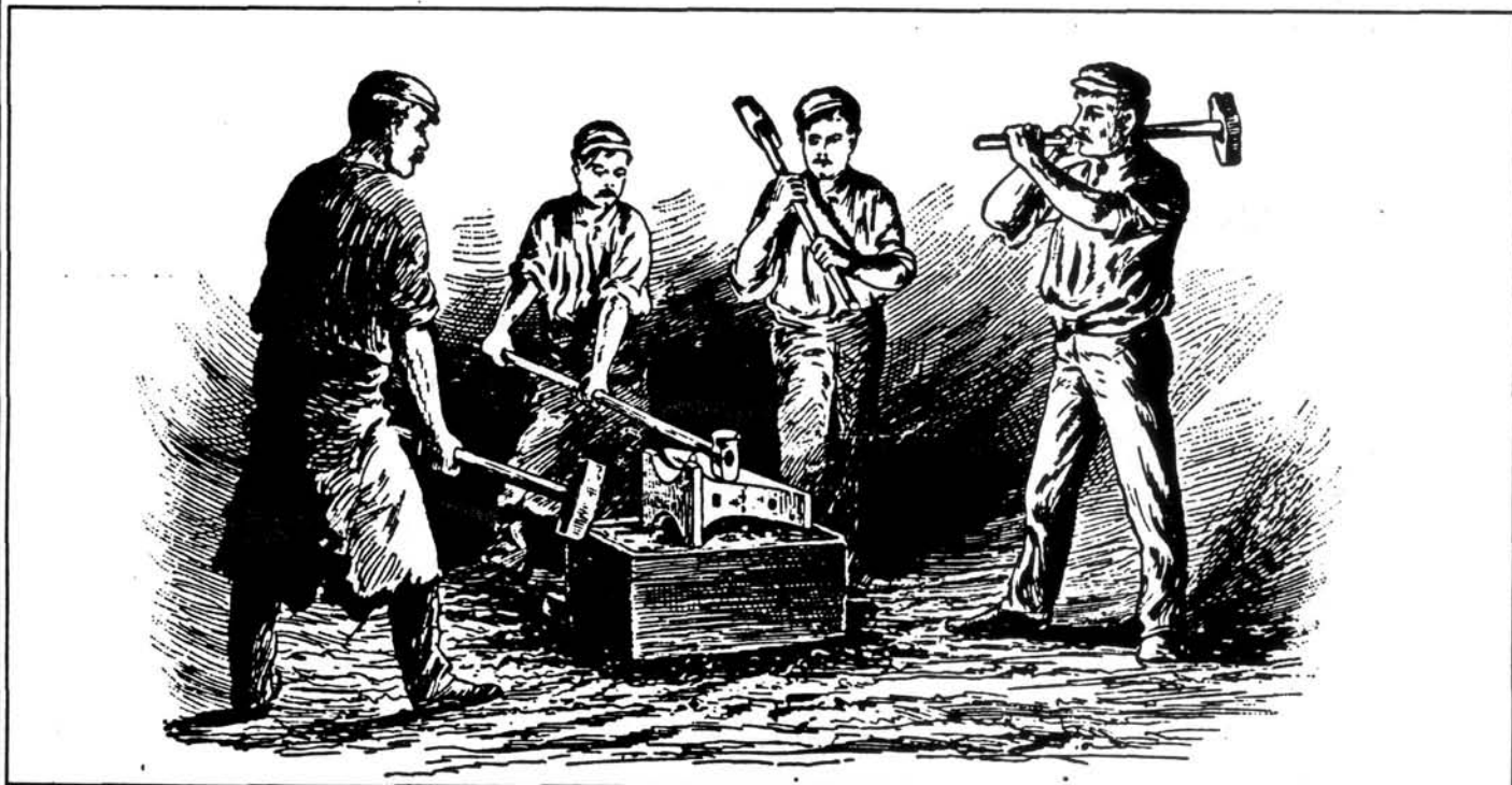
Figure 8 - Finishing Anvil by hand hammering.
