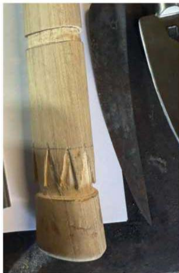
Pics to right: Handle with areas pewter will be poured chiseled out.
