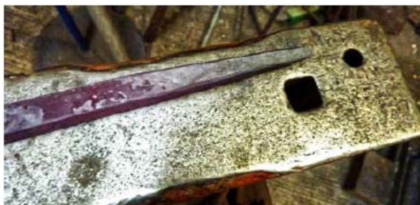
Taper with chamfered corners-
