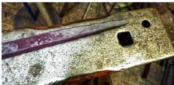
Taper with chamfered corners-
