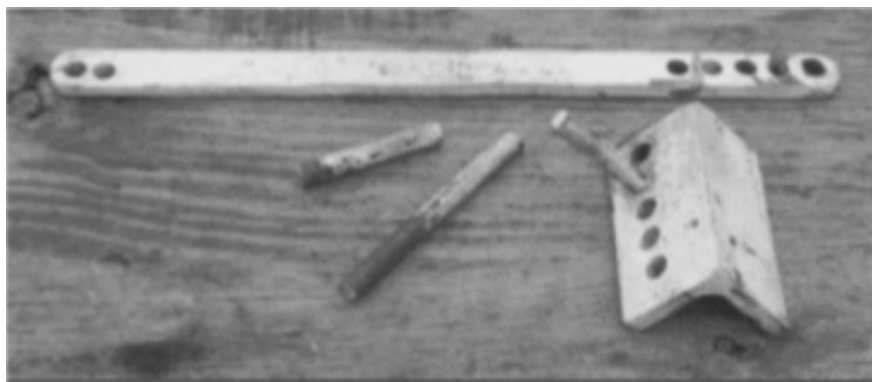
Bender parts, handle, base, three pins
