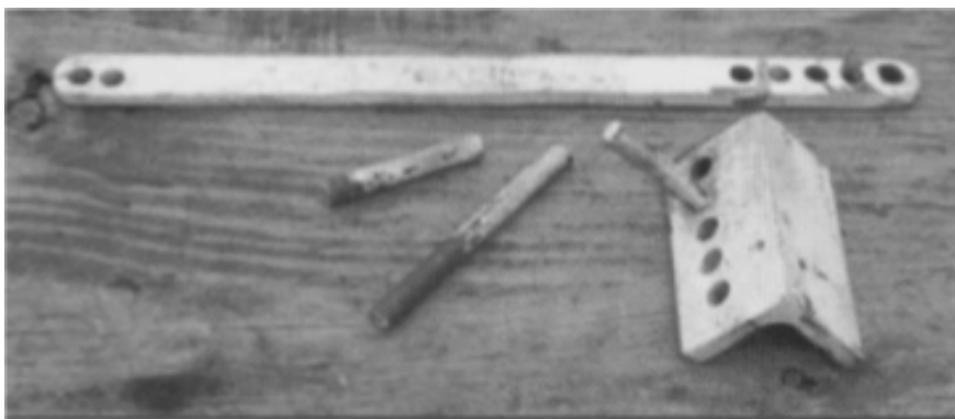
Bender parts, handle, base, three pins
