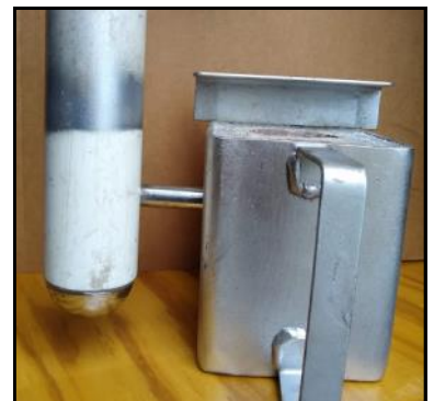
Above photo shows how the PVC pipe, attached ball and 5/8" pin sit inside forge for casting step.
