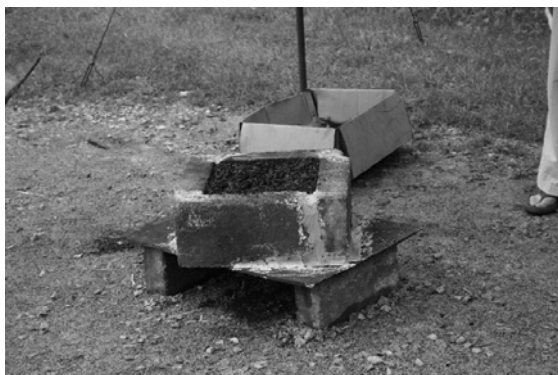
The base for the bloomery furnace: Four cement bricks on an elevated steel plate, the center filled with charcoal fines.
