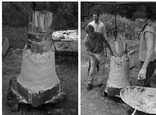
The partially completed clay furnace and Dave and Marshall finishing clay furnace.
