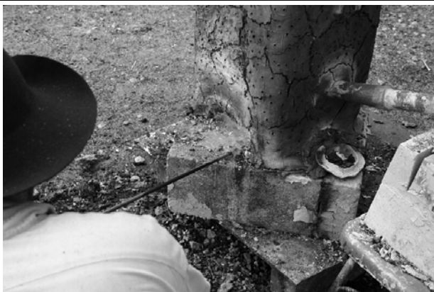
Mike examining the slag running from the furnace
