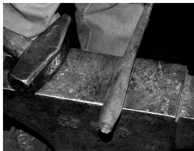
Shaping the handle and starting the loop.
