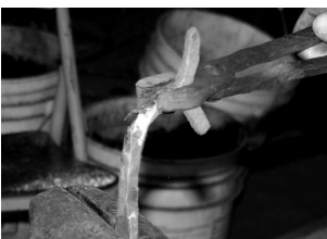
Drawing out bar and bending to draw out tines.
