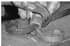
Using a channel-locks to close the collar.)
