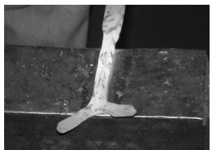
Drawing out bar and bending to draw out tines.
