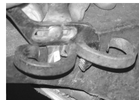
Using a channel-locks to close the collar.)
