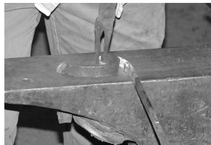
Forming the scroll on the scroll jig.
