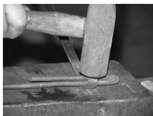
The collar on the mandrel, ready for the final legs to be hammered down.
