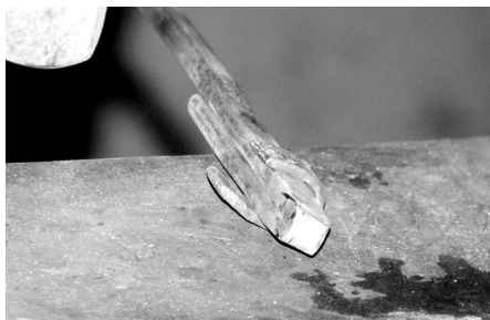
The collar on the mandrel, ready for the final legs to be hammered down.
