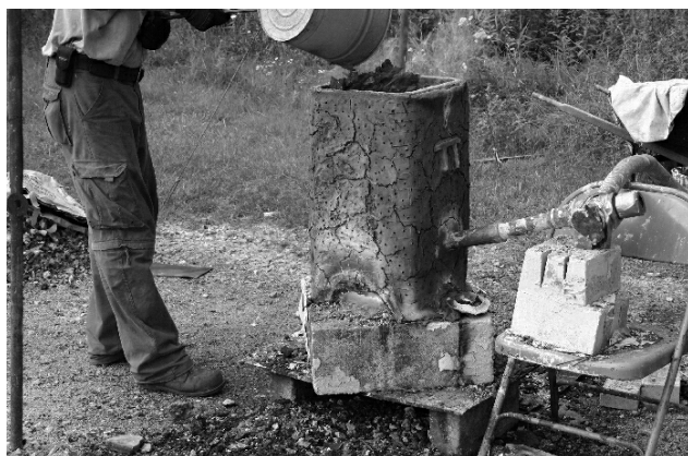
The furnace in blast. Dave charging coal.
