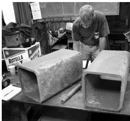
Two 12" flue tiles supplied by Bruce Ringier. Marshall in the back-ground.
