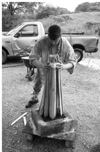
Mike assembling the mandrel (form) for the furnace.
