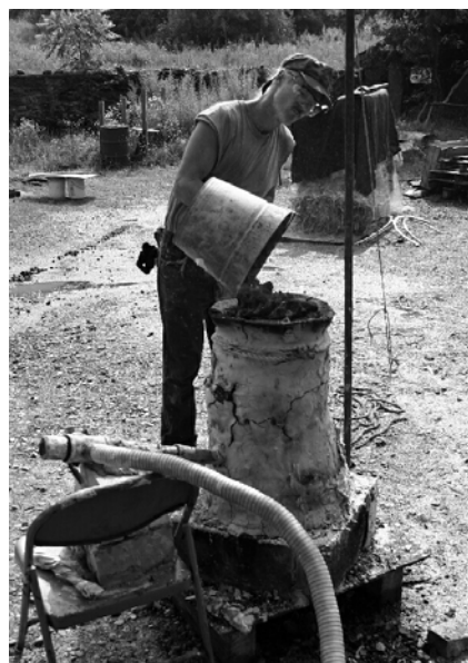
Charging the furnace with charcoal.
