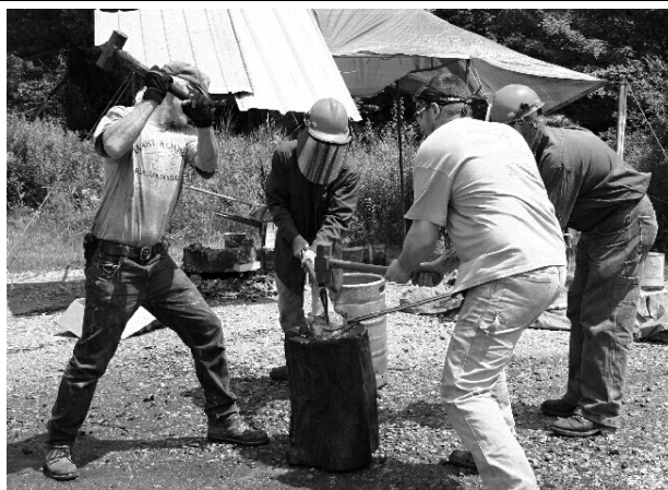
Dick holding the bloom, Marshall holding the axe, while Dave and Mike strike
