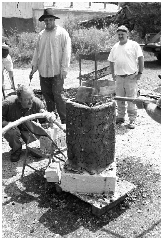
The furnace in blast. Marshall charging ore. Dick viewing the smelt through the sight glass. Mike and three visitors watching.
