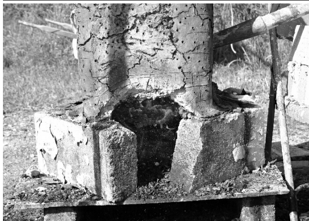
The furnace near the end of the smelt. Half of one brick removed. Bottom of bloom is visible.
