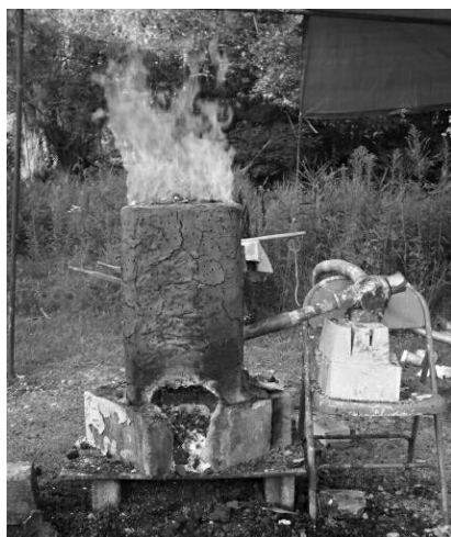
Mike built a wood fire under the bloom, fanned by a second blower, to keep the bloom hot
