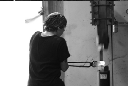
Mike and Dick working the bloom. Beth working the bloom on an air hammer.
