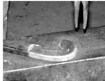
The half-finished C-scroll on the scroll jig.
