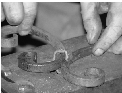
Fitting two C-scrolls in a collar.
