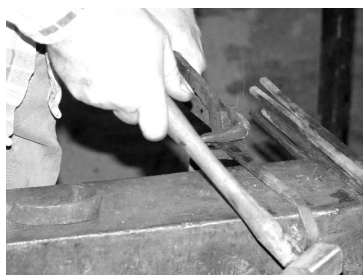
Starting the second scroll over the edge of the anvil. A close-up.
