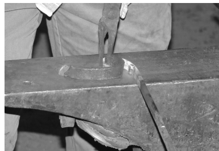
Forming the scroll on the scroll jig.
