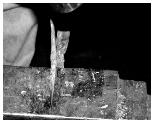
Drawing out bar and bending to draw out tines.
