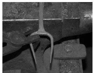
Drawing out bar and bending to draw out tines.
