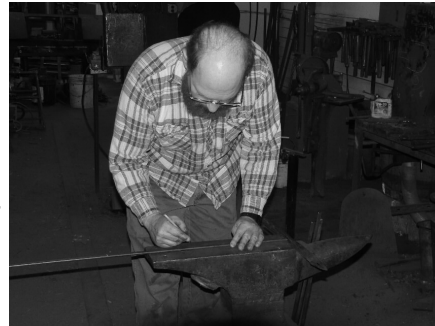
Marking the scroll stock with a soapstone stick.
