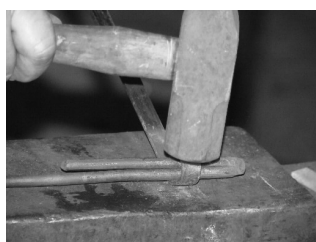
The collar on the mandrel, ready for the final legs to be hammered down.
