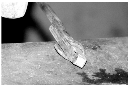
The collar on the mandrel, ready for the final legs to be hammered down.
